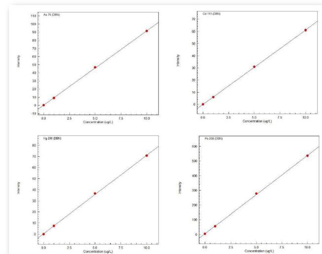
Figure 2: Calibration curves for As, Cd, Hg, and Pb [µg/L]
